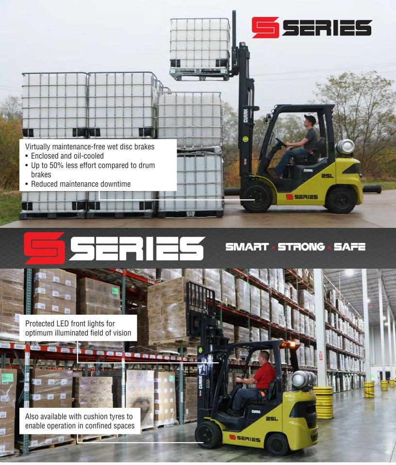
Stylish design – solid construction and greater security and operating comfort for the driver. With the S-Series, we have created a truck that focuses on the needs of the operator more than ever before. The next generation of internal combustion forklifts has arrived – the new S-Series.
