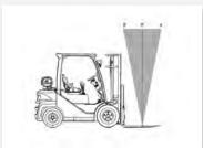
Vertical mast system Automatic tilt lock when upright is in vertical position
